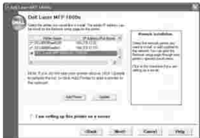
If you do not see your multi-function printer in the list, click Update to refresh the list or click Add Printer to add your multi-function printer to the network. To add the printer to the network, enter the port name and an existing IP address for the printer.
